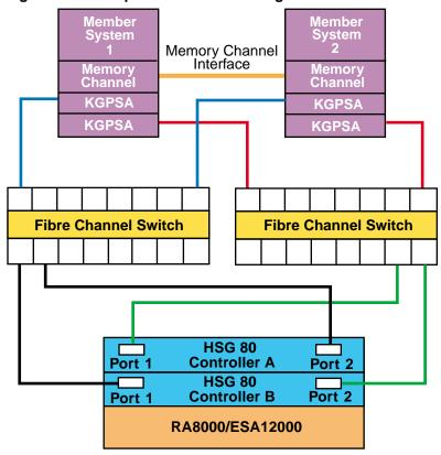
Figure 6-7: Multiple-Bus NSPOF Configuration Number 3
